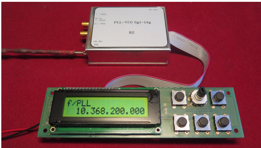
Bild 2 (5355 PLL + DISPLAY-UNI-1) PLL-VCO 0g1-14g-5mW + DISPLAY-UNI-1
